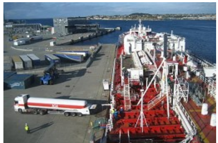
Incorrect parking position for bunker road tanker.
