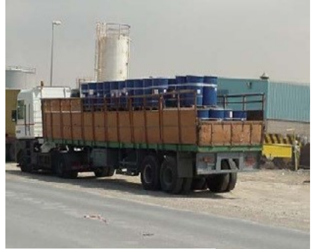
Unsafe Securing Arrangement
