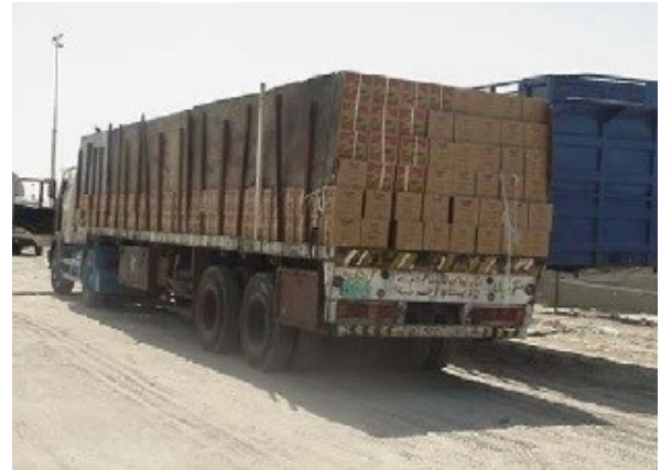
No Rear Side Securing Arrangements
